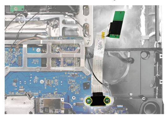
Lift the flexible cable out of the rear housing.
